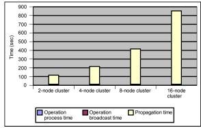
Figure 1. Propagation operation timing results on four clusters.
