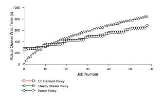
Figure 4. Actual queue wait time, in seconds. All jobs are one minute jobs with two minute walltimes, submitted simultaneously.
