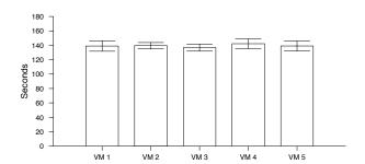
Figure 5. Startup times of 5 VMs (with standard deviation), launched simultaneously, on the Nimbus cloud at the University of Chicago.
