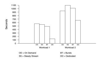
Figure 7. Elapsed time (seconds) of the workload, from submission of the first job to completion of the final job. For the dedicated policy 10 VMs are started prior to submission and run for the duration of the test.
