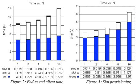
We first timed how long it takes to adapt a node for VM deployment using the Xen balloon driver. We used the the xm mem-set command to reduce the memory in domain 0; on average this took 743.6 ms (SD = 100.5). Restoring the memory includes system checks (e.g., for running VMs) and took 1317.2 ms (SD = 96.5). The kill-all
